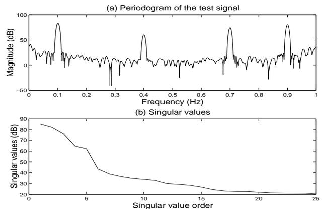
Fig. 2. Periodogram and singular values of a synthetic signal
