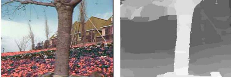
Fig. 1.1: Optimal disparity obtained with a global stereo functional and an efficient graph cuts algorithm (experiment taken from [5]). Such stereo methods depend on (at least) two parameters which it is difficult to estimate. Notice the obvious errors: the house and the sky have the same disparities. On the top-left the disparities of the tree branches and of the sky are mixed up. Global methods are not well adapted to a strong sub-pixel accuracy because they quantize the disparity to avoid a complexity blow up. In this experiment, there are only eight disparity levels.
