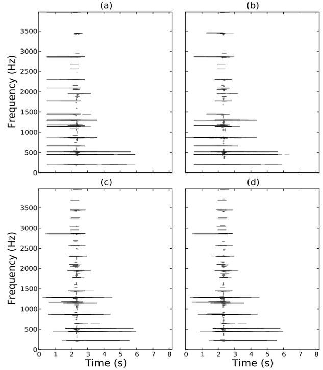
**Fig. 2.** Energy distributions of a bell sound decomposed by MP and LOMP algorithms. Left: original signal decomposition at 20 dB SRR with 8 MDCT basis with MP (a) and LOMP (c). Right: decomposition of the same signals shifted in time by 100 samples with MP (b) and LOMP (d).
