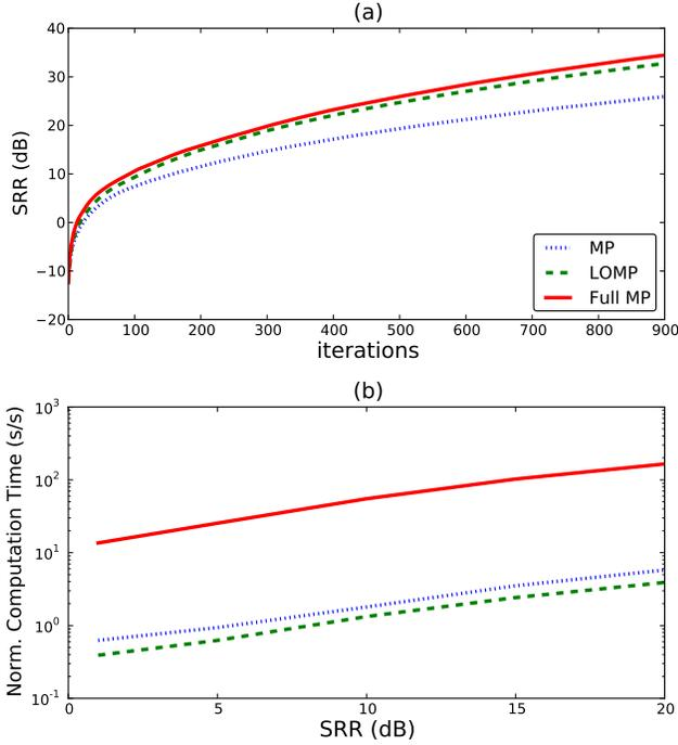
**Fig. 1.** Comparison of (a) : convergence rates and (b) : Complexities in computational time , for MP , FullMP and LOMP decomposition of 4096 samples of orchestra signal over a dictionary of 3 MDCT basis (32,128,512).
