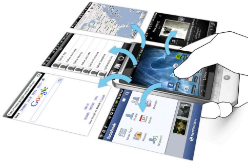
Figure 9. An example of an implementation of JerkTilts for switching among applications.
