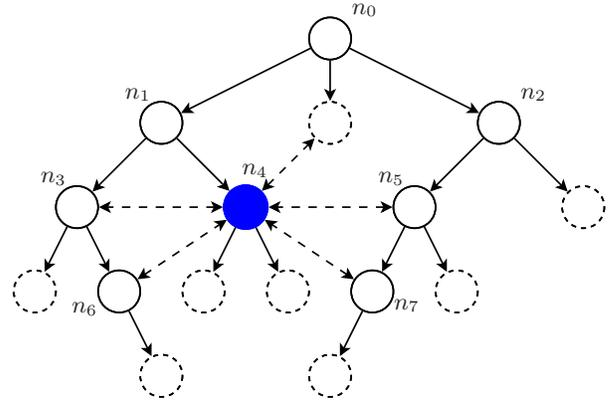
Figure 2. Example of directed graph of an ABCD overlay (all nodes, solid lines) for one description. Solid border represents active nodes. Neighbouring relations for node  $n_4$  (dashed lines) are also represented. Here,  $\mathcal{B}_4 = \{n_5, n_6, n_7\}$ ,  $\mu(n_4, n_5) = \mu(n_4, n_7) = n_0$ , and  $\mu(n_4, n_6) = n_1$ . Being  $h(n_0) = 0$  and  $h(n_5) < h(n_7)$ , we designate as foster parent for  $n_4$  the node  $n_5$ .
