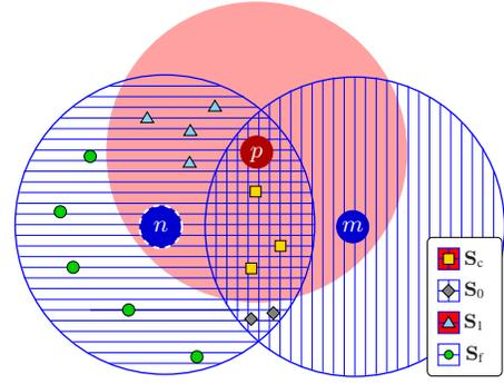
Figure 1. Sets  $\mathbf{S}_c$ ,  $\mathbf{S}_0$ ,  $\mathbf{S}_1$  and  $\mathbf{S}_f$  with respect to node  $n$ . Here  $N_c = 3$ ,  $N_0 = 2$ ,  $N_1 = 4$  and  $N_f = 5$ . Only nodes  $n$ ,  $m$  and  $p$  are active. The pattern in the background of the nodes' transmission area is parallel lines for description  $d_0$  and solid for  $d_1$ .
