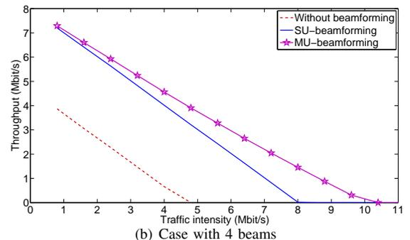
Fig. 6. Mean user throughput vs. traffic intensity.
