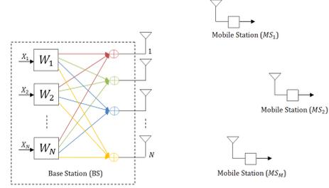
Fig. 1. Block diagram of the MU-beamforming system.
