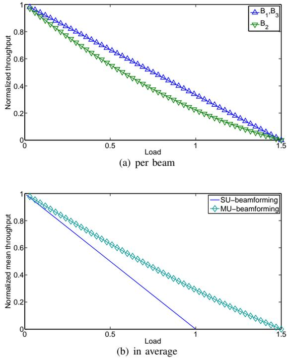
Fig. 3. Normalized user throughput with MU-beamforming with 3 beams.
