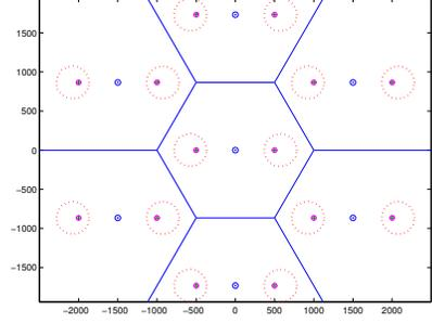
Fig. 3. Network of heterogeneous cells. Macro-stations are identified by the symbol  $\odot$ , small-cell stations by  $+$ . The first ring around each  $+$  gives the minimal distance to small-cells. Each small-cell coverage area (given by equation (16)) is in dotted lines.
