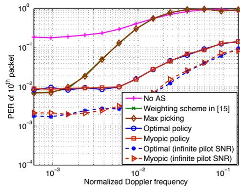
Fig. 2. PER vs normalized Doppler frequency ( $f_m T_{\text{pkt}}$ ) for the 10<sup>th</sup> packet for 4-states channel model with data SNR = 20 dB.
