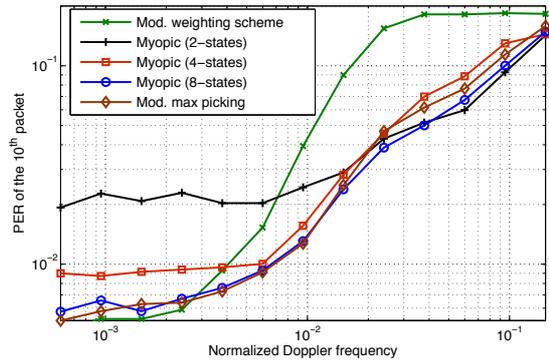
Fig. 3. PER vs normalized Doppler frequency for the heuristic methods for the 10<sup>th</sup> packet with data SNR = 20 dB.
