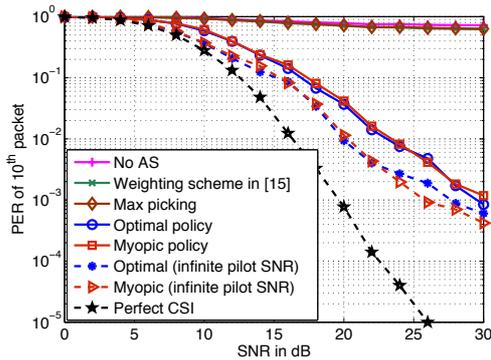
Fig. 1. PER vs SNR for the 10<sup>th</sup> packet with  $\kappa = 4$  and  $f_m T_{\text{pkt}} = 0.02$ .
