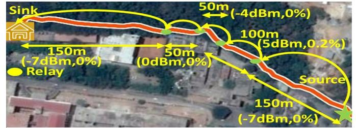
Fig. 4. Real deployment along a long trail using OptExploreLimLearning with iWiSe motes,  $\xi_o = 100$ ,  $\xi_r = 1$ : five nodes (including the source) are placed; link lengths, transmit powers, and % outage probabilities are shown; the plot shows variation of end-to-end loss probability with inter-packet duration for periodically generated packets from the source
