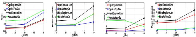
Fig. 3. Model-based results for  $\xi_o = 10$ : mean cost per step, mean power per link, mean outage per link and mean placement distance (steps) vs.  $\xi_r$  for the four algorithms: OptExploreLim, OptAsYouGo, HeuExploreLim, and HeuAsYouGo. The node power in the HeuAsYouGo algorithm was taken to be the same as the mean node power with the OptExploreLim algorithm. The unit of  $\xi_r$  is actually mW, but here it is shown in dBm.
