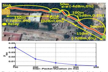
Fig. 4. Real deployment along a long trail using OptExploreLimLearning with iWiSe motes,  $\xi_o = 100$ ,  $\xi_r = 1$ : five nodes (including the source) are placed; link lengths, transmit powers, and % outage probabilities are shown; the plot shows variation of end-to-end loss probability with interpacket duration for periodically generated packets from the source
