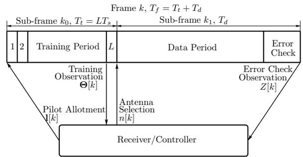
Fig. 1. Sequence of operations in frame  $k$ .
