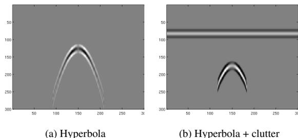
**Fig. 2:** Simulated B-scan
